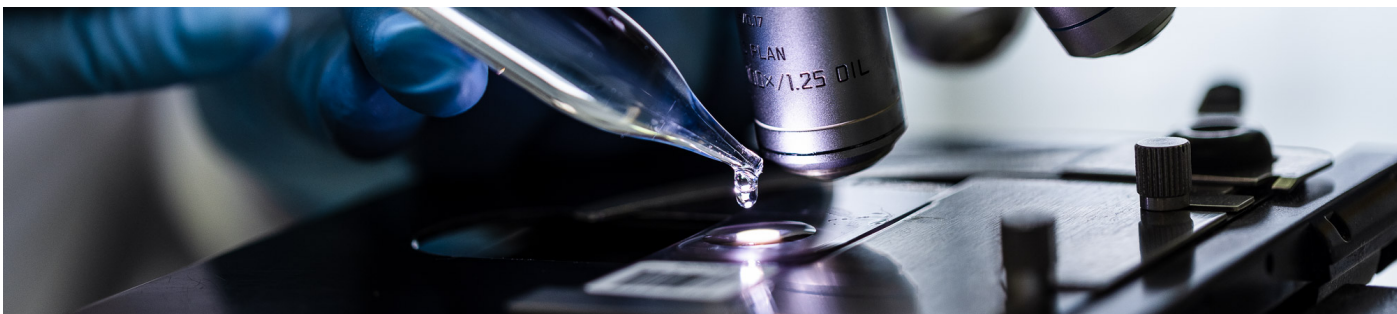
Drop deposit of immersion oil
