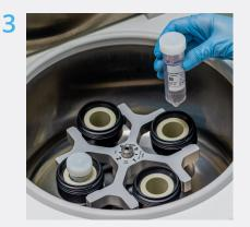
Centrifugation is safely performed thanks to robust prolypropylene tubes.
